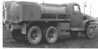
CCKW Fuel Truck, 750 gallons, 2 1/2 ton 6x6. 1941 photo
