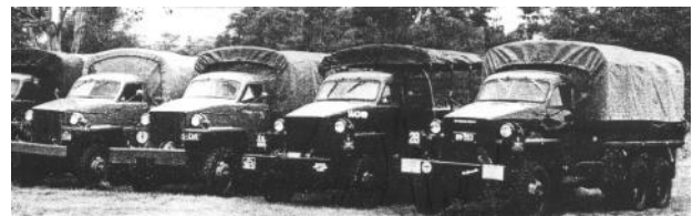
The photo directly above is of a line-up of Studebaker trucks 'in their day'; the 3 rd veh from the right is fitted with a self recovery winch, identifiable by the cut-away section in the middle of the front bumper bar.
